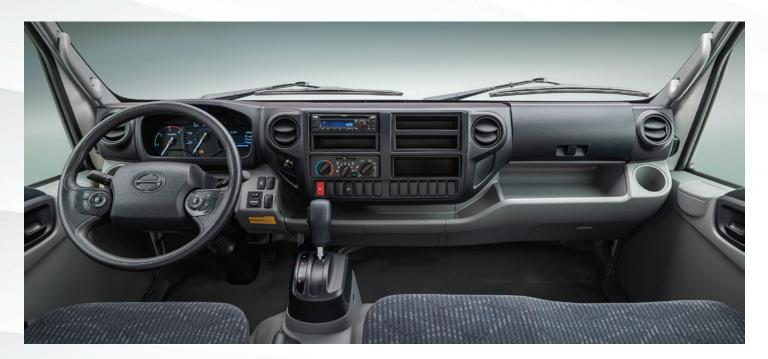
NEW interior design equals more functionality! A new gauge cluster featuring a 4.2" LCD multi-information display for easier vehicle monitoring and a new Aisin 6-speed HD automatic transmission with a gear hold feature, especially useful in steep incline situations.
